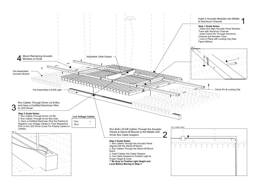
\*\*NOTE: To be installed by a certified electrician based on the codes of the region of installation. Fishtnk Inc. recommends two separate junction boxes for low voltage and high voltage wires. To comply with electrical code. A licensed electrician can install as appropriate.
